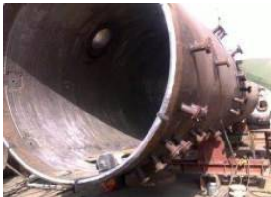
Fig 2.2 Stainless Steel Cladding
